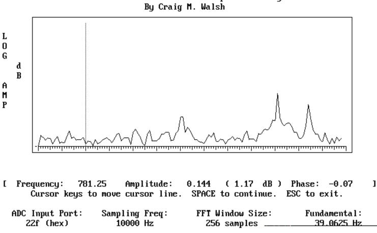
Above is a spectrum diagram of the PK-2 sidetone with a piezo output.
