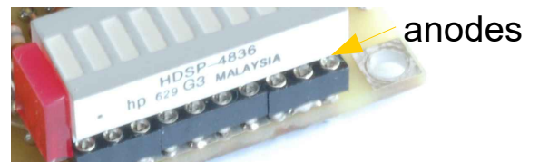
Detail of LED array orientation
