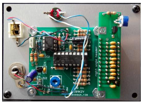
5) Finally (after testing it out per the board assembly manual) mount the front panel in the case using the four x black 4-40 machine screws.
