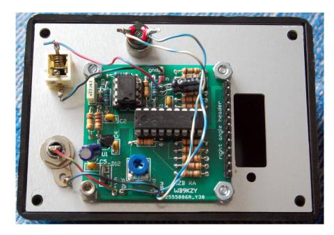
4) Mount the daughter board on the straight header as shown with the front of the LED array flush with the front panel. The 3mm LED may have to be adjusted to fit. Solder the header and LED to the daughter board.
