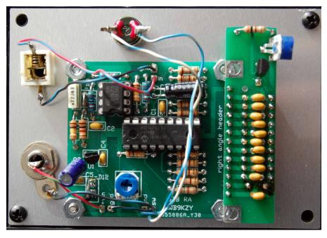
5) Finally (after testing it out per the board assembly manual) mount the front panel in the case using
