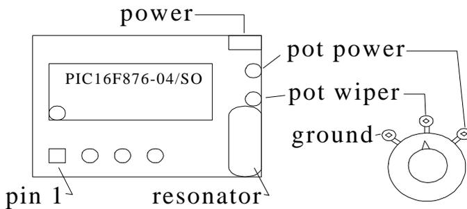
the left. Pin 1 of the MegaPK corresponds to pin 1 of the keyer chip that the MegaPK is replacing. The MegaPK circuit board is roughly 5/8 inch by 7/8 inch.
