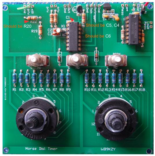
Prototype version 1 board with some errors. Production version 2 bare boards at right.
