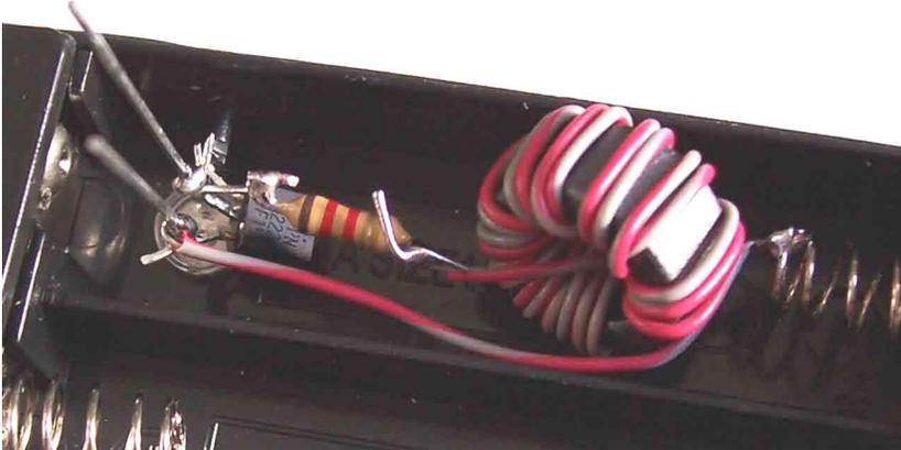
17) clip the leads, check the connections and insert the battery:
