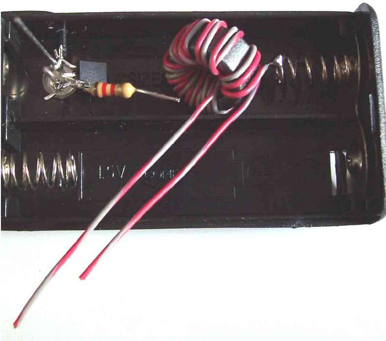
15) solder the shorter toroid wire to the 1.2 kohm resistor:
