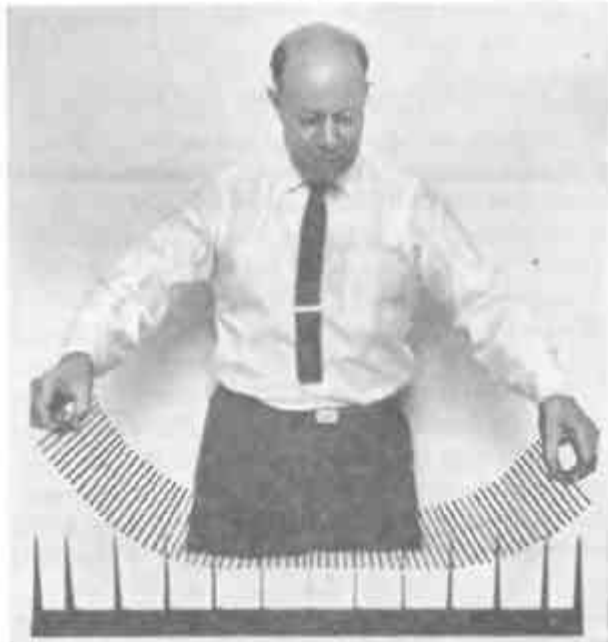
Figure 2-7. To mount the machine lift the wave structures and lower it into the notches of the bearing plates.
