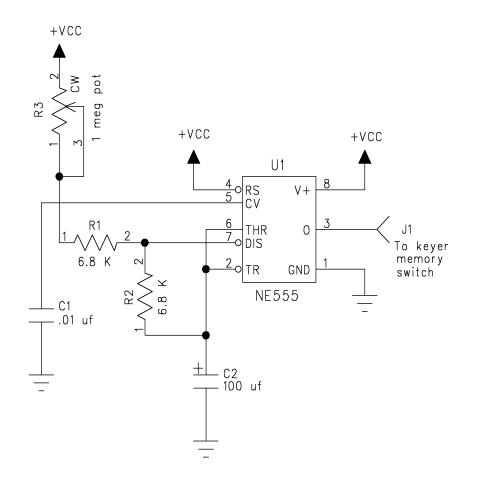
This circuit can be used with the Island Keyer to provide a beacon timer.
